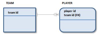
**Note:** Standard IE notation does not include rounded corners on entities. Rounded entity corners are an IDEF1X symbol included in IE notation to help ensure compatibility between methods.
