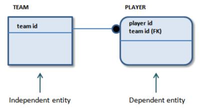
Dependent entities are further classified as existence dependent, which means the dependent entity cannot exist unless its parent does, and identification dependent, which means that the dependent entity cannot be identified without using the key of the parent. Because PLAYERs can exist if they are not on a TEAM, the PLAYER entity is identification-dependent, but not existence-dependent.
