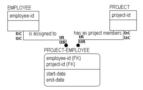
Cascade indicates that all instances of PROJECT-EMPLOYEE that are affected by the deletion of an instance of PROJECT should also be deleted. Restrict indicates that a PROJECT cannot be deleted until all instances of PROJECT-EMPLOYEE that have inherited its key have been deleted. If there are any left, the Delete is restricted.
